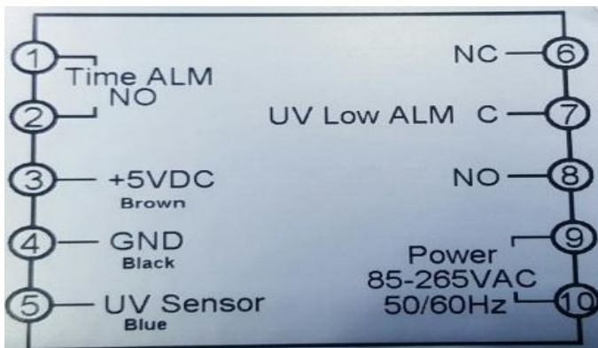
Fig. 2 Connection Diagram of UV Radiometer 6
