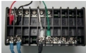
(2) Connection method (Top: Voltage, Bottom: Current)
