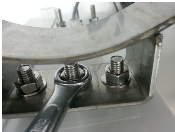
Fig5-②. Insert washer and nut, tighten the nut using a spanner.
