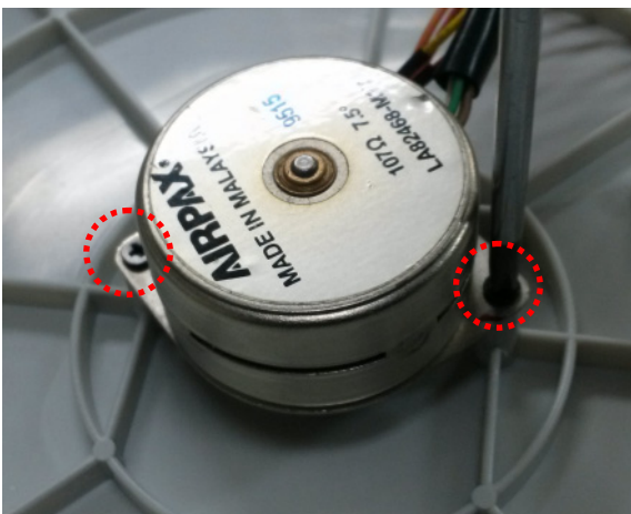
Fig13-④. Separate the stepping motor screws at back side of panel.
