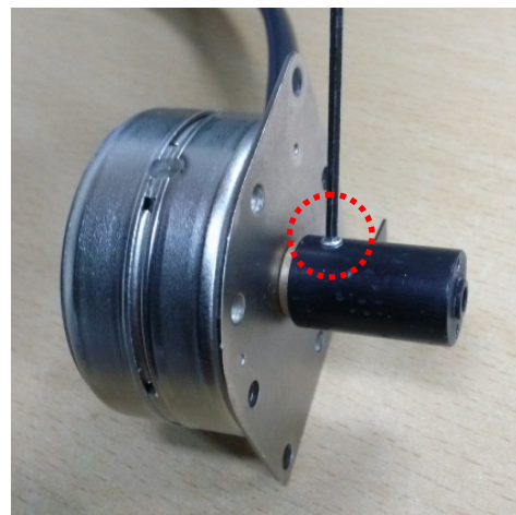
Fig13-⑤. Separate the supporter of hand of indicator with hexagonal wrench.
