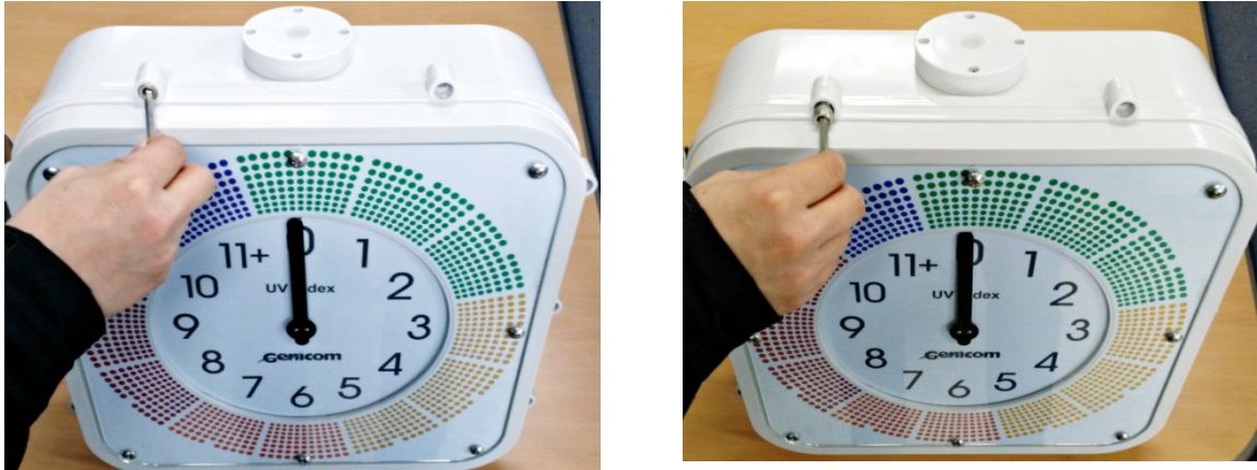
Fig.15-① Detaching the cover from the main body
