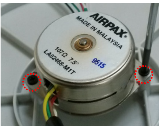
Fig14- ④. Separate the stepping motor screws at back side of panel.
