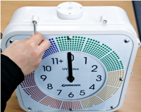
Fig14-①. Unfasten the screw the hexagonal screw by using hexagonal wrench and open front panel
