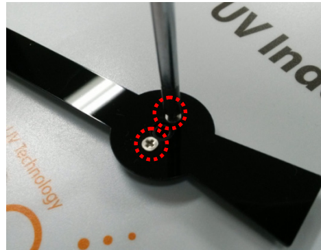
Fig14- ③. Separate the cross head screws from hand of a indicator.
