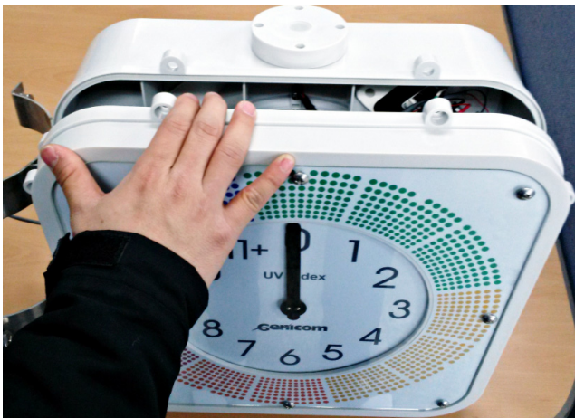
Fig.15-② Opening front panel cover
