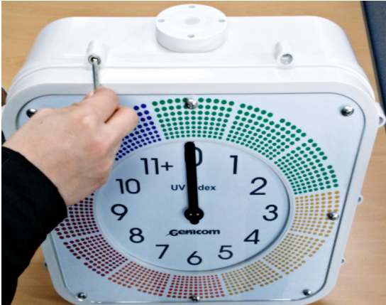
Fig13-①. Unfasten the screw the hexagonal screw by using hexagonal wrench and open front panel
