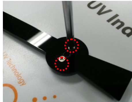
Fig13- ③. Separate the cross head screws from hand of a indicator.
