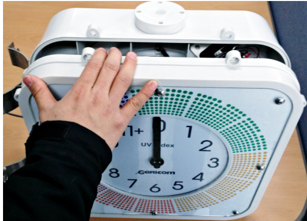
Fig13-①. Unfasten the screw the hexagonal screw by using hexagonal wrench and open front panel
