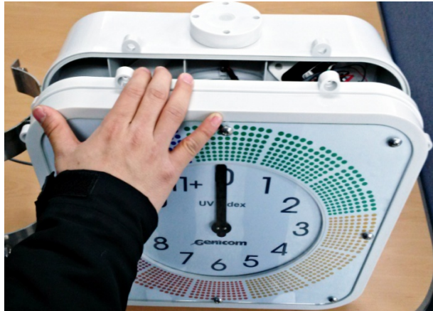
Fig14-①. Unfasten the screw the hexagonal screw by using hexagonal wrench and open front panel
