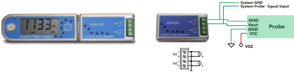
Fig 5. External Input 0~5V Wiring diagram
