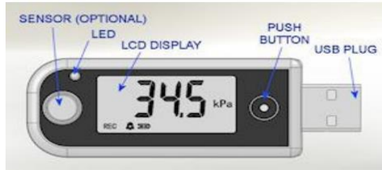
Fig 4. Each part functionality of Datalogger
