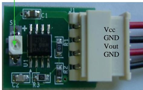
Fig. 2 Application module of UV Sensor
