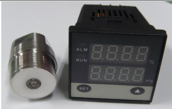
Fig. 1 UV Radiometer 6 (Size of Display : 48 × 48 × 107mm)
